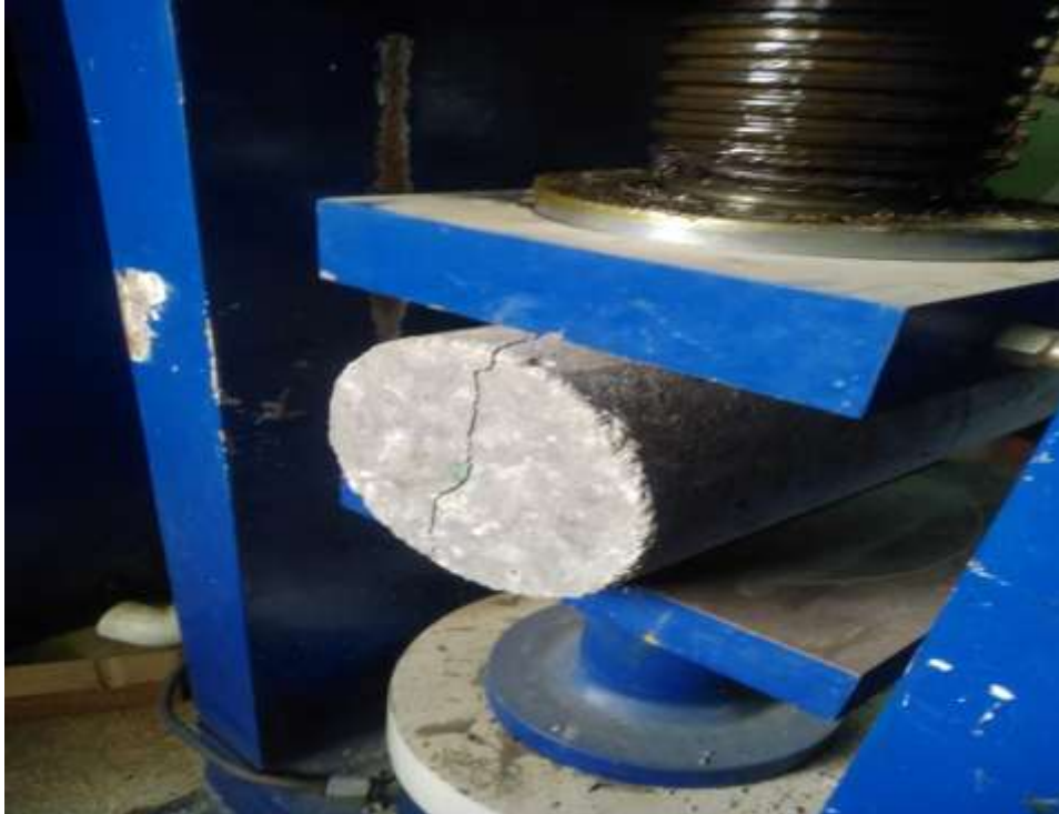
FIG 3.2: Split Tensile Test of Cylinder
