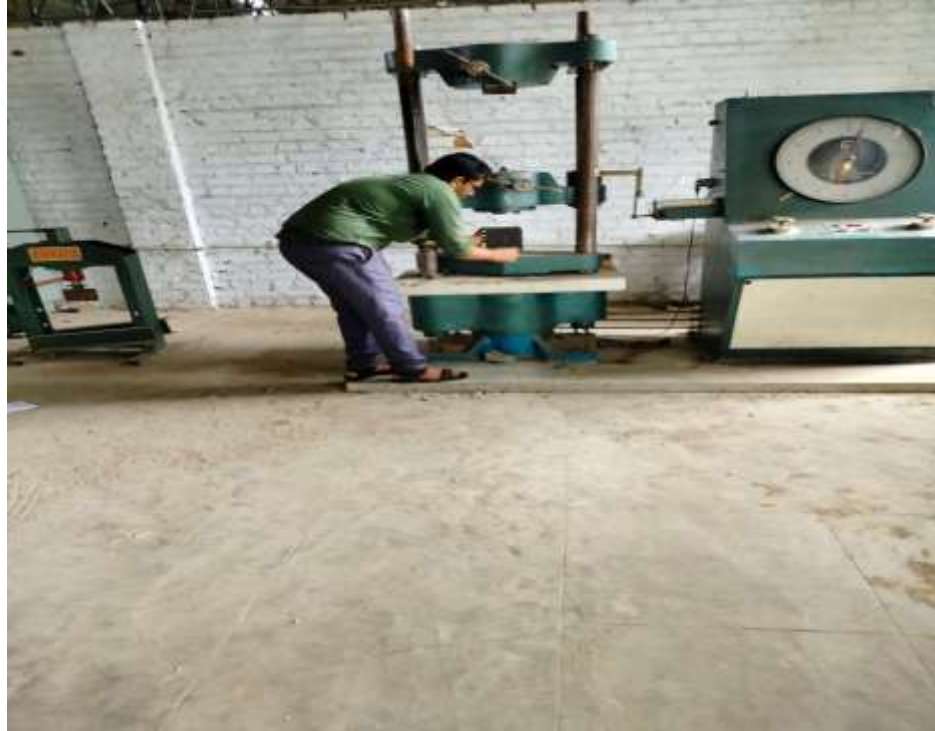
FIG 3.1: Compressive strength testing of Cube
