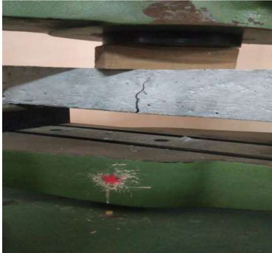
FIG 3.3: Flexural Strength Test of Prism
